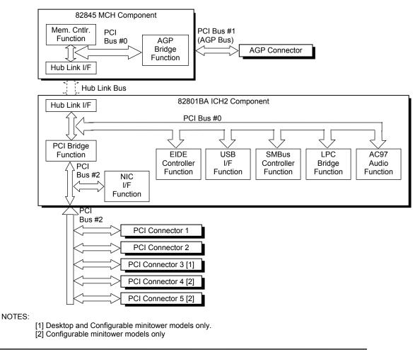
4-2 Compaq Evo and Workstation Personal Computers Featuring the Intel Pentium 4 Processor Figure 4-1. PCI Bus Devices and Functions
